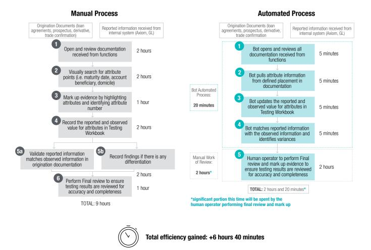
The side-by-side comparison of manual and automated approaches to transactional testing of 25 transactional samples demonstrates how automating the process gains efficiencies and saves an estimated six hours and 40 minutes as compared to the manual process. The automated process increases efficiency as the human operator only performs value-added tasks, such as documentation confirmation, marking up the selected attributes in the source
